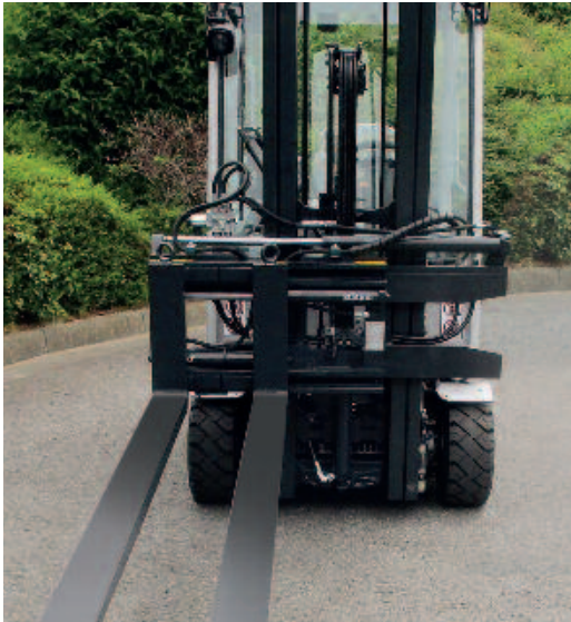
Sideshifter for container loading combined with special fork positioner
