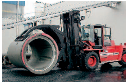
Tilting concrete pipe clamp
