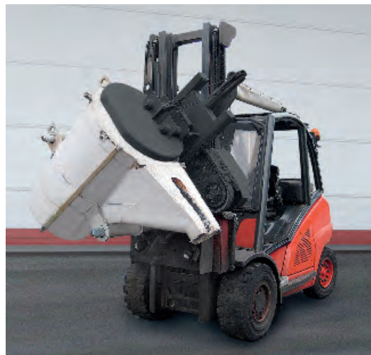
Side tipper with sideshift and hydraulic lid opener
