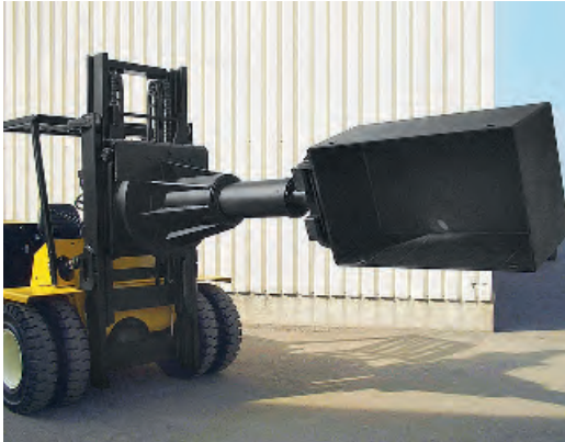
Charging device with hydraulically lockable box
