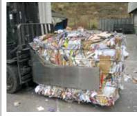
The waste management and recycling industries focus on the disposal and recycling of various materials. Materials such as waste paper and cardboard packaging, plastics and textiles are regularly transported in the form of bales. Metals are usually collected in bins and containers and are later supplied to processing operations. Bale clamps, pivoting fork clamps, fork clamps, scrap grapples and rotators are required for handling
