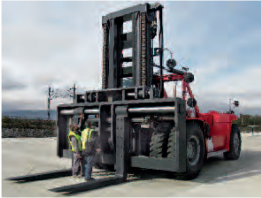
Fork positioners - load capacity 55,000 kg / 1,200 mm
