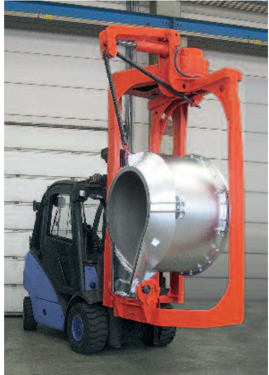
Ladle tipper with ladle
