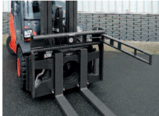
Rotator with lateral support arm; manually adjustable, foldable and mountable on either side
